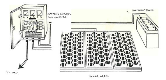
The Milyering Centre has dual circuit systems which are powered by solar panels. Solar panels convert light energy into electrical energy which is stored in large battery banks. A conventional electrical supply is then generated by devices known as inverters. Inverters convert direct current (d.c.) voltage from batteries into alternating current (a.c.) power at the standard household voltage of 240 volts, 50 Hertz.
