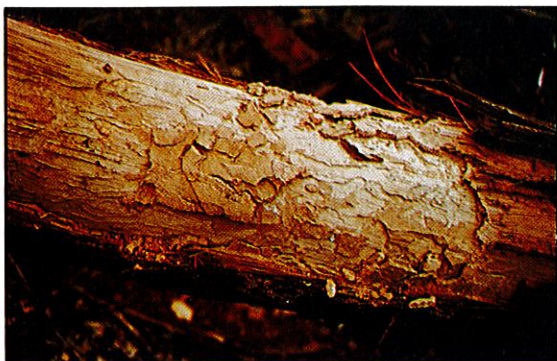
Figure 1 Bardi attack on sapwood of recently felled jarrah. This attack may be prevented by storage under water spray or by removal of bark.
