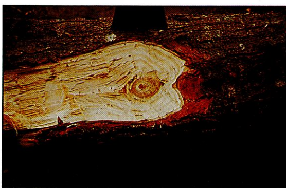
Figure 22 Knot in radiata pine. This is an "intergrown knot".
