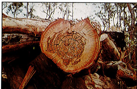
Figure 6 Cubical rot in jarrah.
