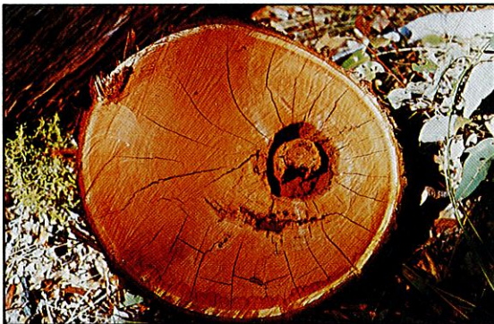
Figure 19 Cross section of jarrah log showing "off-centre" heart with associated rot.
