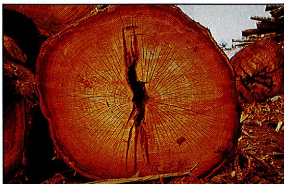
Figure 28 Heart shake in karri, with associated rot.
