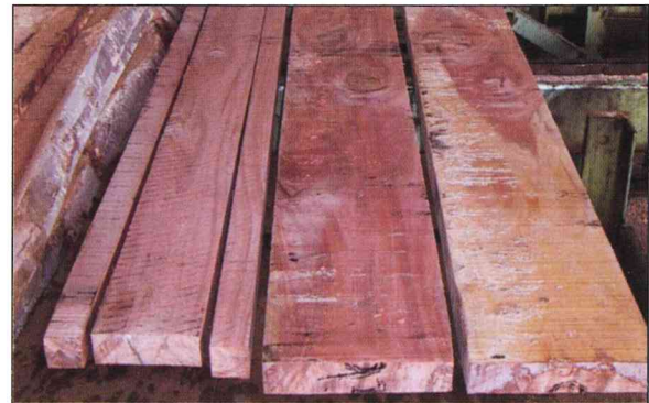
Saligna boards after milling.
