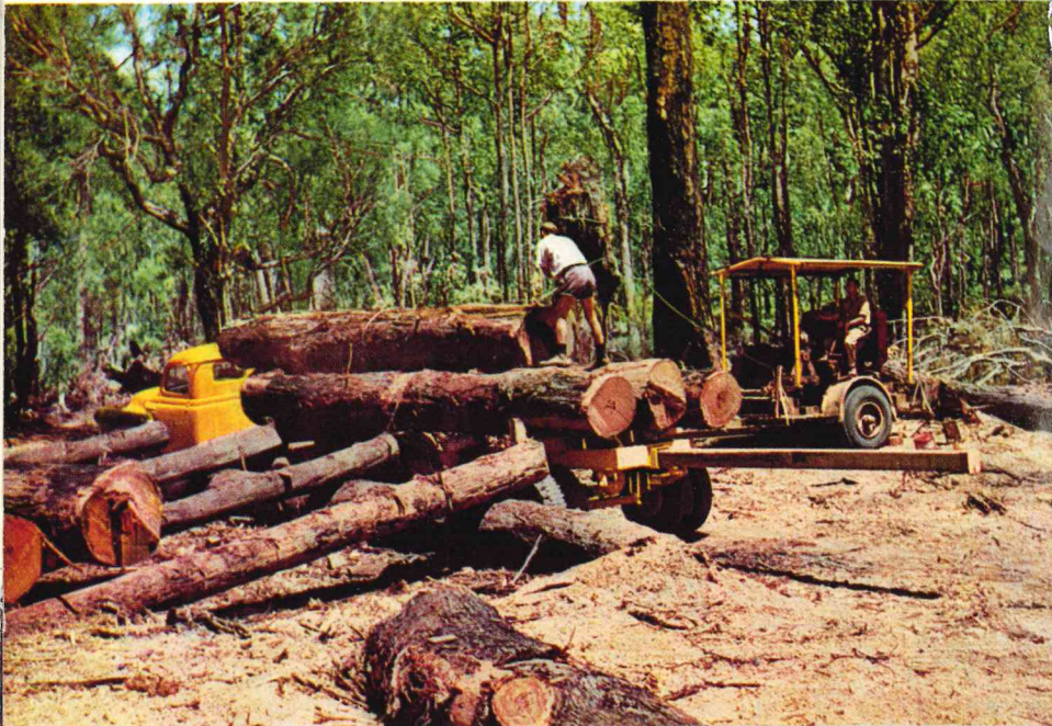
Winch hauling logs onto a truck for cartage to mill. A jinker attached to the pole protruding from the rear of the truck is used to carry extra long logs.
