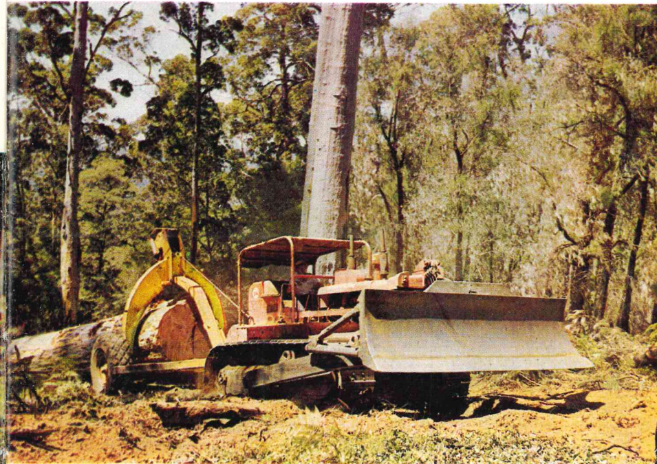
Snigging (or hauling) with a crawler tractor and logging arch.
