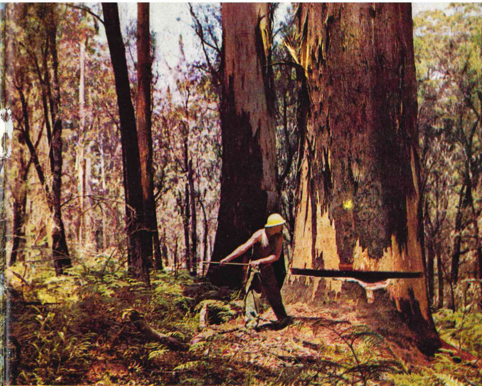
Cutting a "scarf" to direct the fall of the tree.
