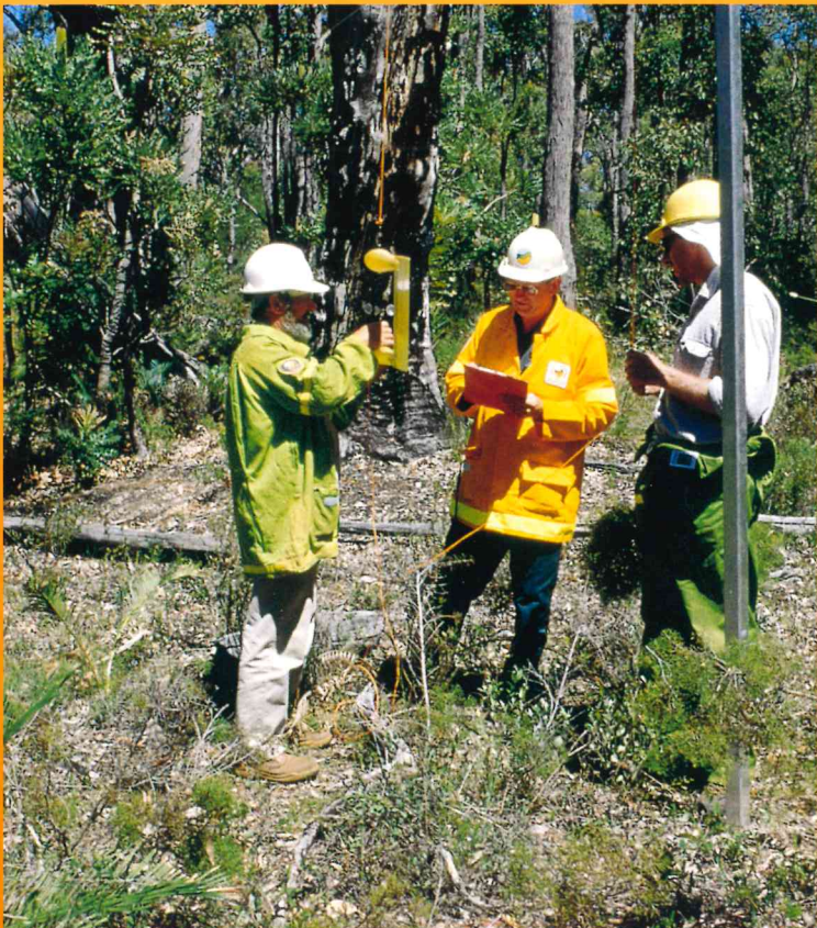
Burn Managers measure forest fuel weights that are used to calculate fire spread and intensity for planned burns. Photo - Lachlan McCaw
