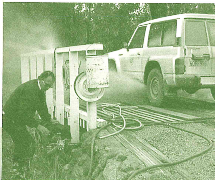
A washdown station used to prevent the spread of Phytophthora fungi.
