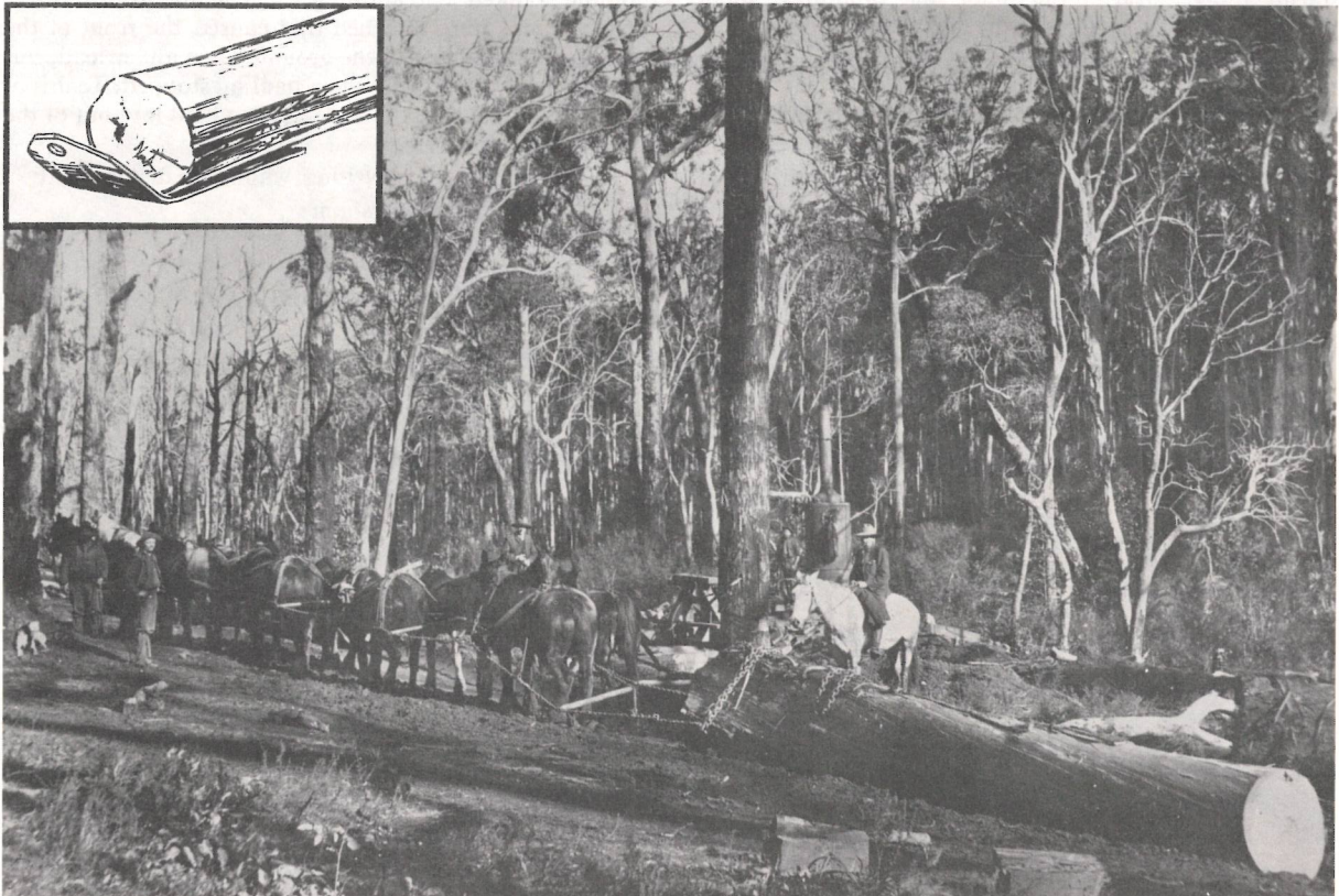
Animal Power: Horse team snigging log. Inset in top left of picture shows the type of steel sled used to reduce friction at the nose of the log.
