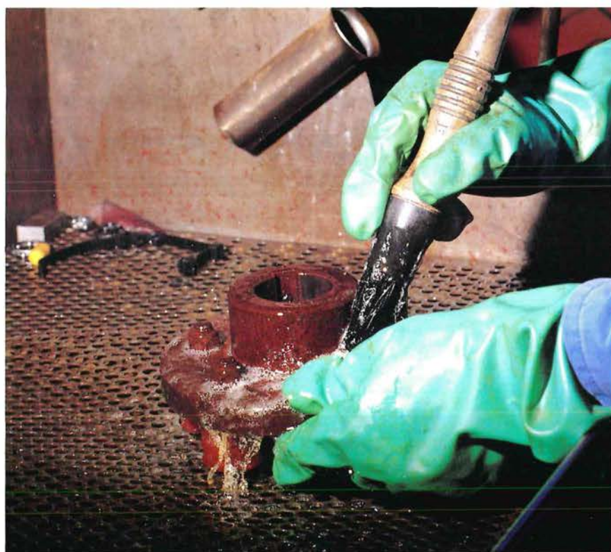
Below: Testing the industrial degreasing value of eucalyptus oil in a workshop at Alcoa's Kwinana Refinery.
