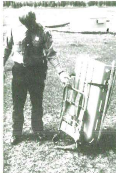
Two piece Ferno-Washington stretcher mounted to rucksack frame, Grand Teton National Park. (This type of stretcher has subsequently been introduced to several W.A. National Parks.)
