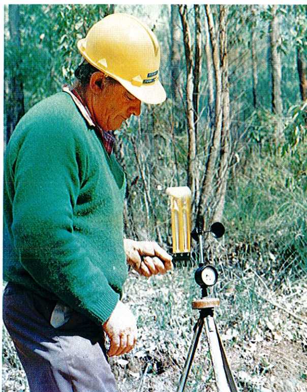
▲ A hygrometer measures wind speed during an experimental fire lit by a research team to collect data on fire behaviour. (Tom Leftwich)
