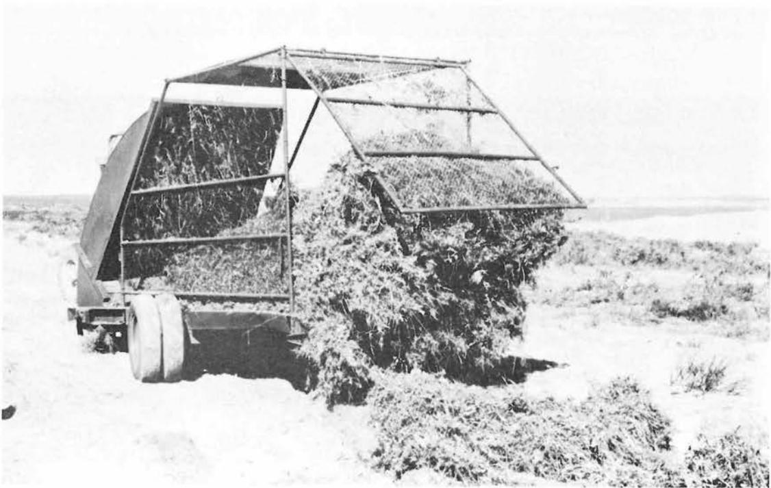
PLATE 4. Harvested material being unloaded from the Forage Harvester onto an area to be brushmatted.
