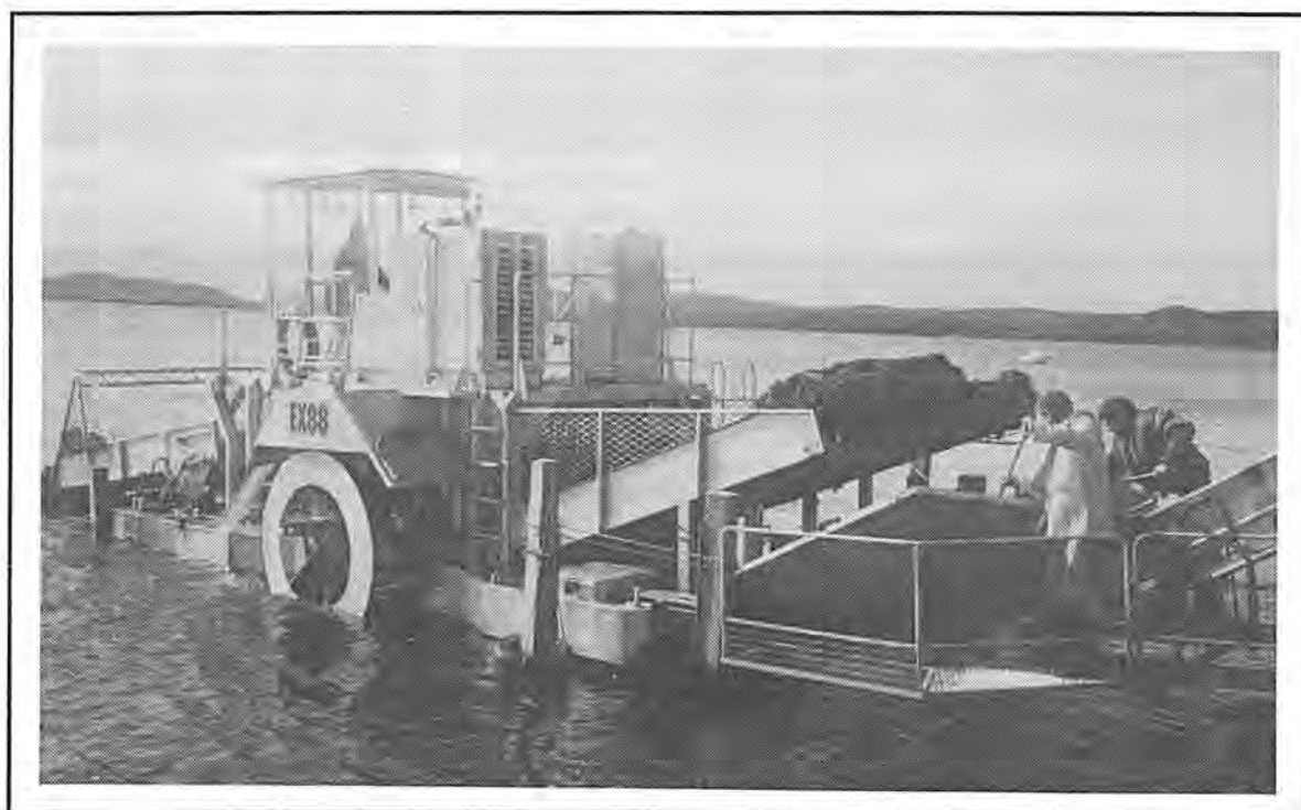
Algae harvesters are used to remove accumulations of macroalgae from Princess Royal Harbour.
