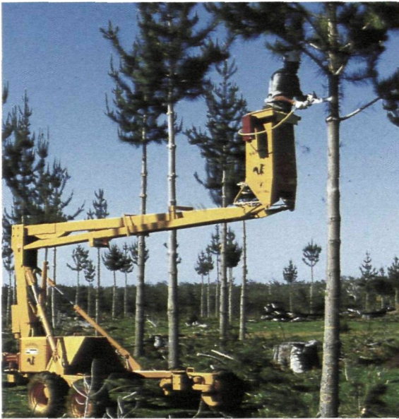
Trees must be pruned to produce saleable timber and to enable reasonable growth of pasture beneath. Machines, such as this specially modified 'Squirrel', have been developed.
