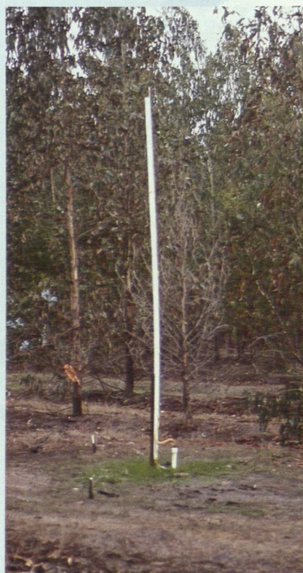
Groundwater pressures 3m above ground in a discharge site planted to blue gums. More planting in the recharge area is required to remove the pressure.
