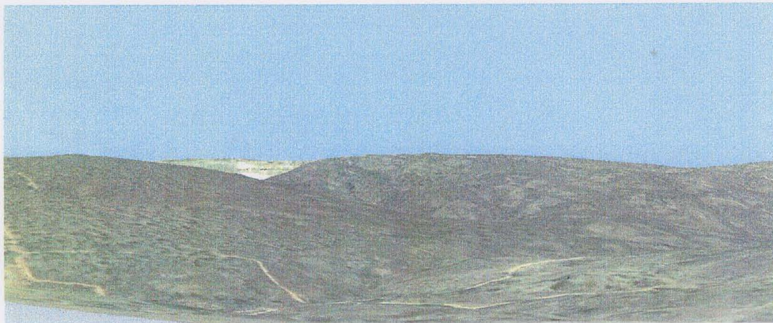
Digital Orthophoto image draped over Digital Elevation Model (DEM) data depicting the visual Impact on 'Teewana' from digital analysis of DEM for equivalent Photo #5. Orthophoto source imagery flown January 2003
