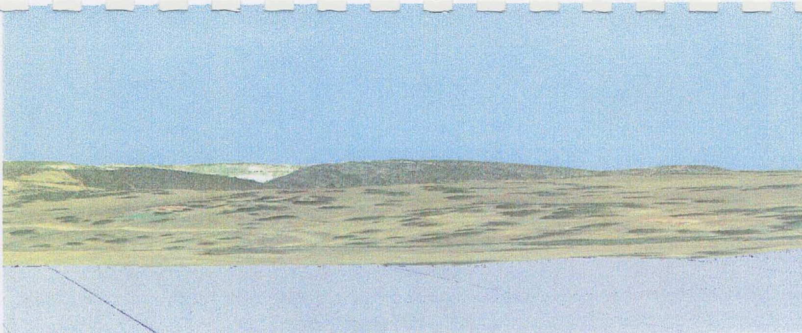
Digital Orthophoto image draped over Digital Elevation Model (DEM) data depicting the visual impact on 'Teewana' from digital analysis of DEM for equivalent Photo #2. Orthophoto source imagery flown January 2003
