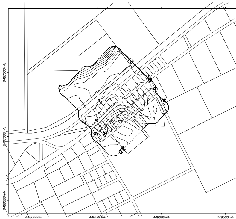
Figure 3-8. Depth to groundwater after 30 years (in metres, contour intervals are 0.5 m) for tree planting simulation
