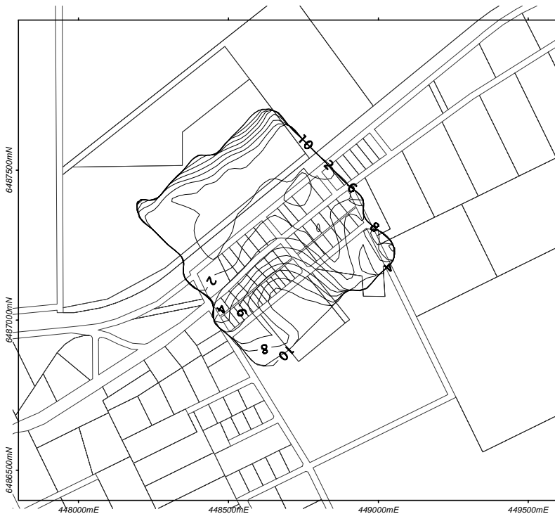
Figure 3-4. Depth to groundwater after 30 years (in metres, contour intervals are 1 m) for 'do nothing differently' simulation
