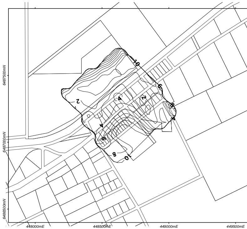
Figure 3-5. Modelled region with management options (simulation area in the centre; the circular objects in a line from south-west to north-east through the centre represent pump locations; adjacent light grey lines represent the simulated drain; dark areas south-east and north-west of pumps represent tree planting areas; boundary scales are in metres; top of map is north)
