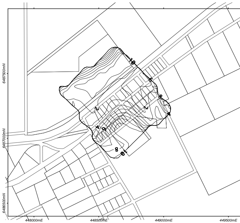
Figure 3-7. Depth to groundwater after 30 years (in metres, contour intervals are 1 m) for drainage simulation
