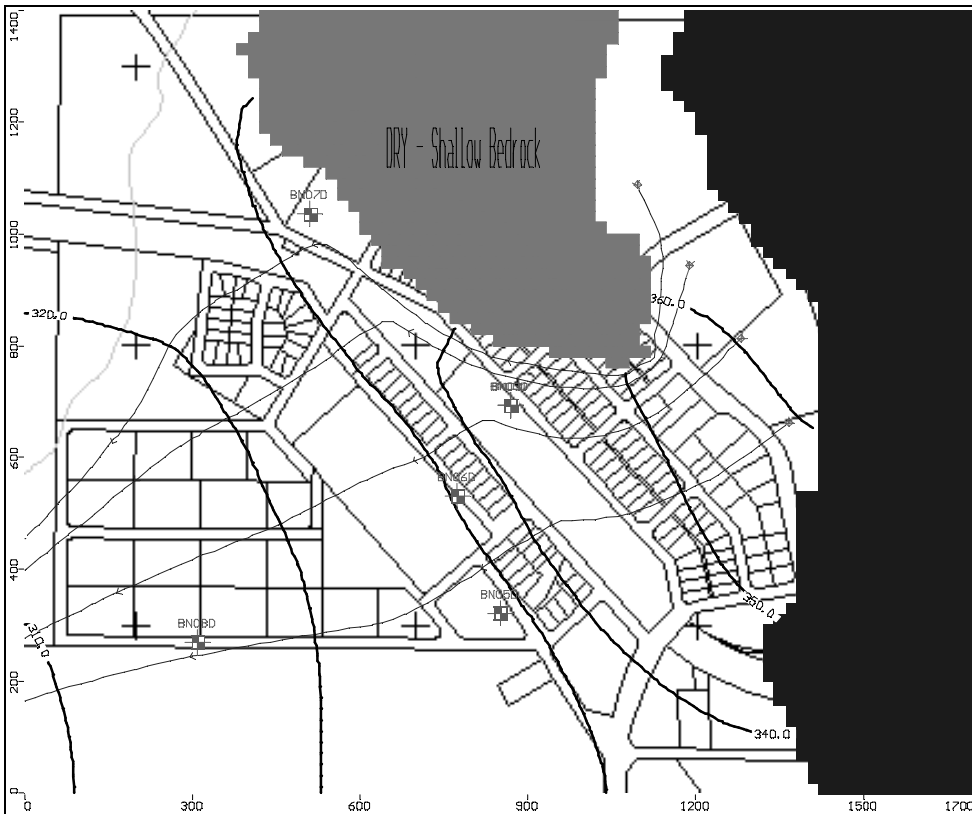
Figure 3-4. Shallow groundwater levels in metres above AHD and travel paths for the calibrated model (boundary scales in metres, top of map is north)
