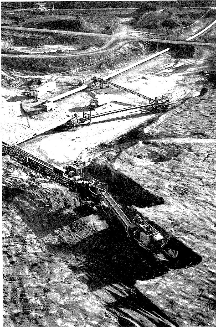
Figure 29. Mining operations at Del Park South, showing a Dosco Continuous Miner loading ore onto an overland conveyor; mobile crusher and overburden stockpiles in background.
