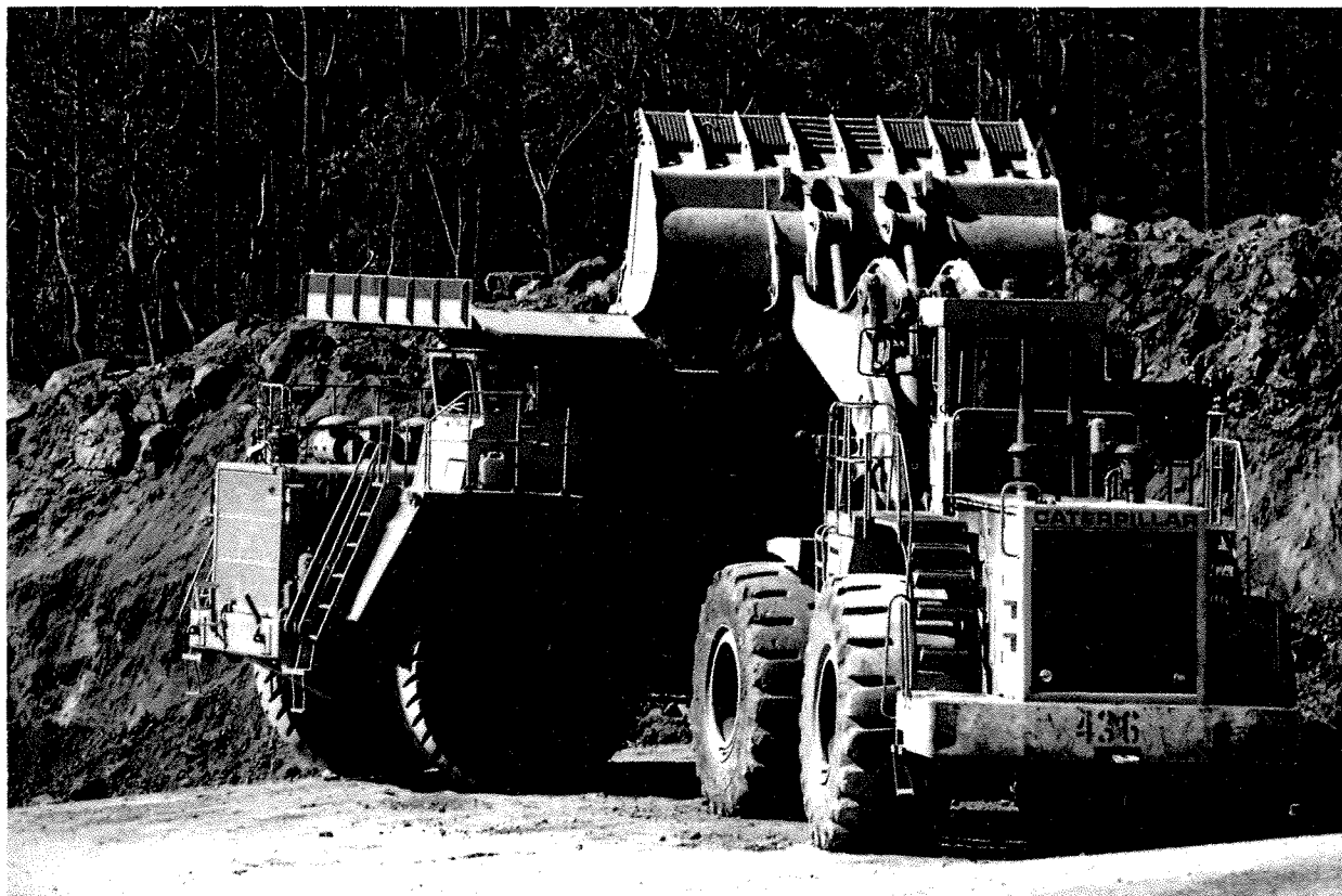
Figure 28. Front-end loader and haulage truck in action at a mine face (Alcoa).
