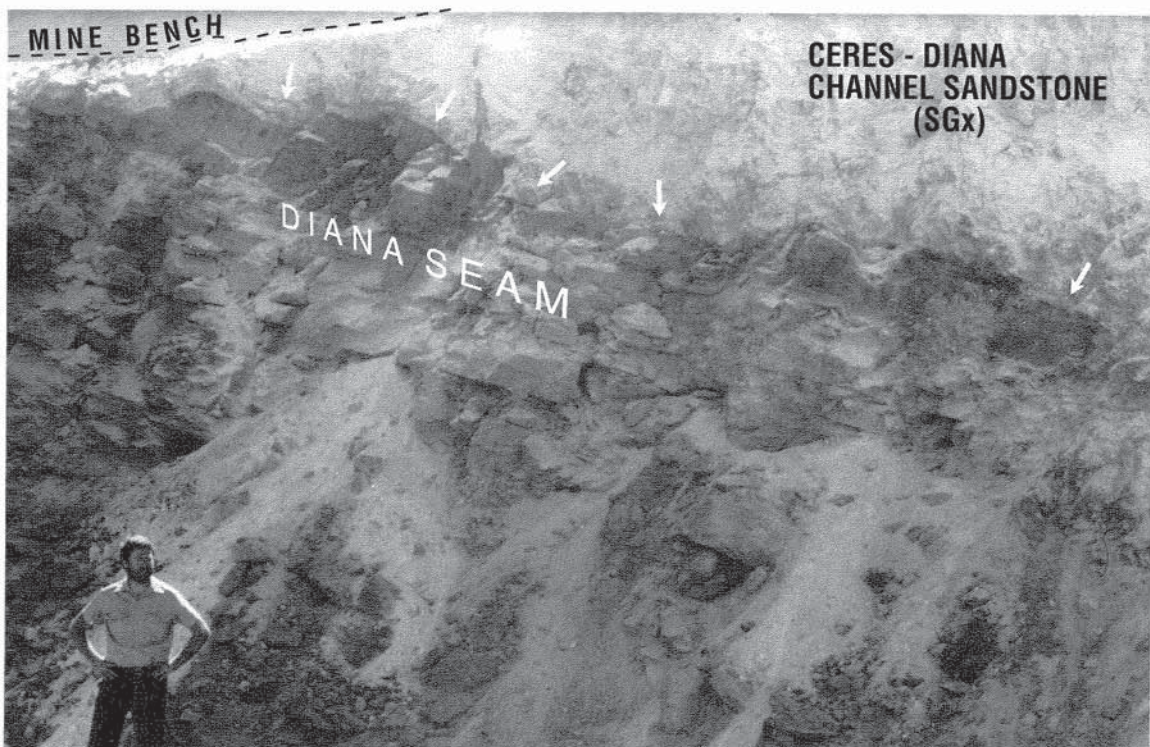
Figure 11. Channel sandstone showing erosive basal contact cut into the Diana Seam; Muja Opencut
