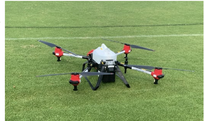
This large commercial drone used for mosquito control weighed approximately 67kg, could carry a payload of 30kg and can treat up to 16ha per hour. Photo – City of Bayswater.
