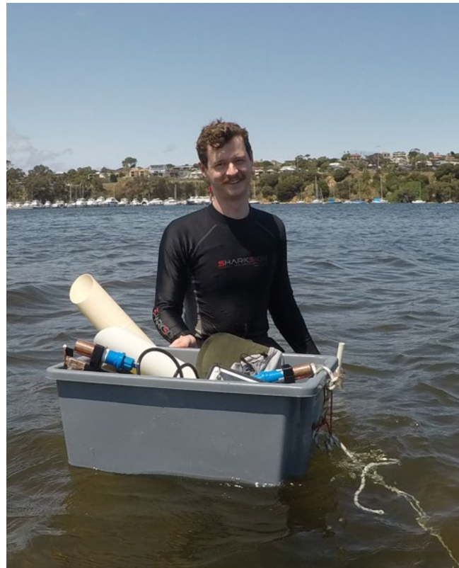
Peter Howie from DBCA installing light loggers into the Swan River at the Rocky Bay site. The light loggers monitor light quantity throughout the season to ensure the seagrass is receiving enough light to photosynthesise efficiently. An important aspect of ensuring we obtain fantastic light data is maintaining these devices in-situ. The 'adopt a logger' program gives volunteers the opportunity to care for and maintain these loggers throughout our seagrass season aiding DBCA in monitoring overall seagrass health. Other volunteer positions assist in monitoring seagrass quadrats in the rivers and in the lab. Photo – Jarra Chapman.
