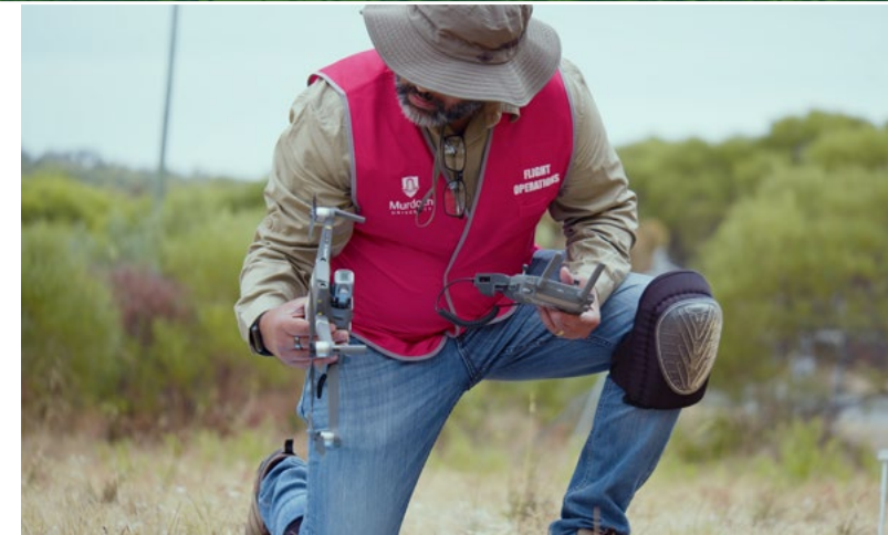
The drone being used for this weed mapping research is low-cost and small. This one weighs less than a kilo, at the time was around $2,500 and doesn't need a licence to operate, meaning that this new technology could be within reach of community groups. Photo – Dannon Wu.
