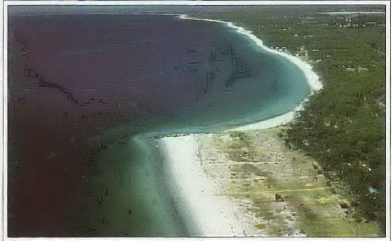
Figure 17. Foredunes are eroded down-drift of the groyne, and the peppermint woodland occurs directly behind the beach (mid to background). Sand accumulation up-drift of the groyne is resulting in foredune species becoming established. Siesta Park, Geographe Bay. (photo: S. Chape)
