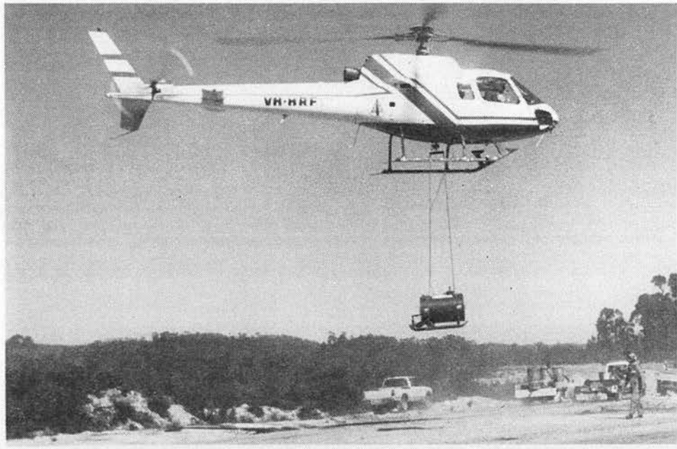
FIGURE 1. HELITORCH IGNITION OPERATIONS
