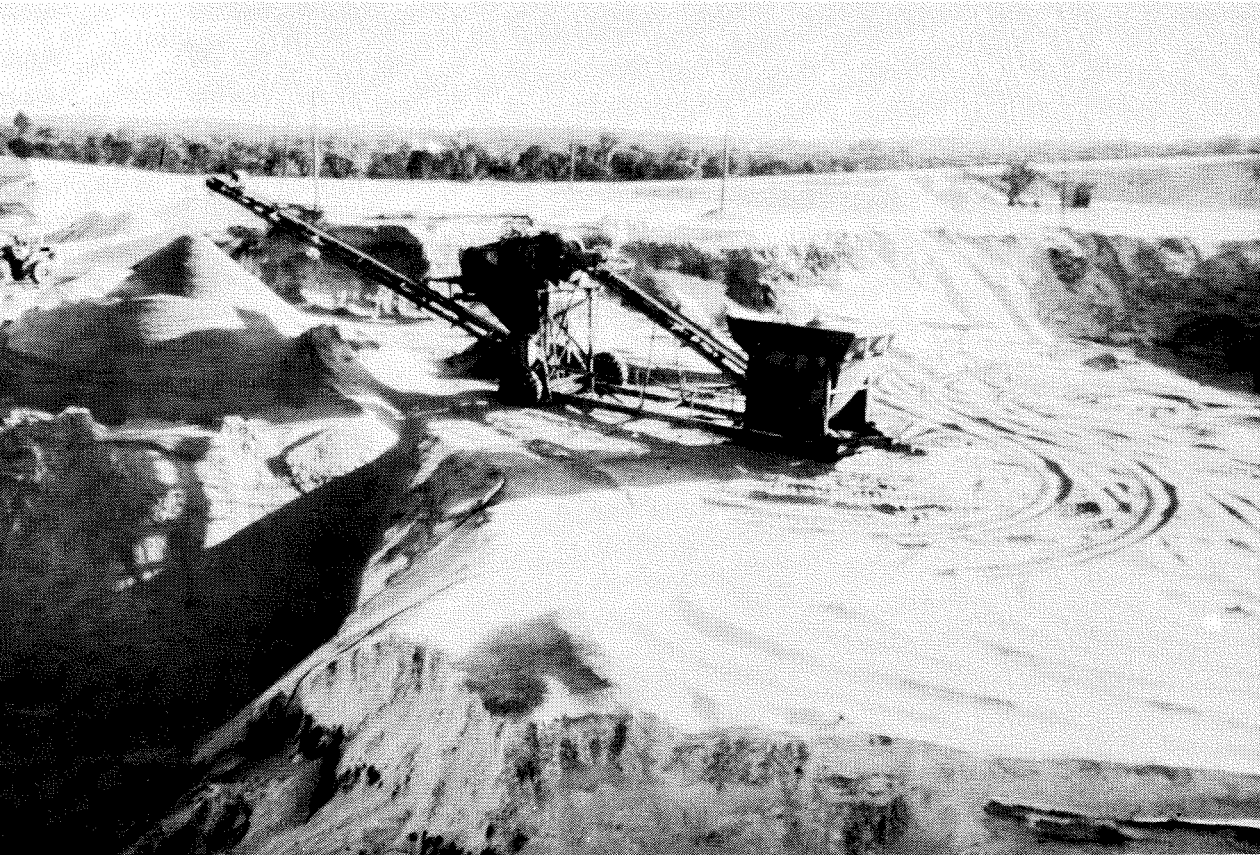
View of Readymix sand pit at Jandakot showing mobile screening plant and stockpiles.
