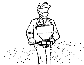
Hand granule sprayer Effective reach: 5 ~ 8 m Outlet capacity: ~ 4 kg/min
