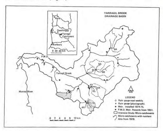
Fig. 1. Yarragil Brook Drainage Basin southeast of Perth, Western Australia. Locations of nutrient monitoring Catchments, weirs and rain gauges.
