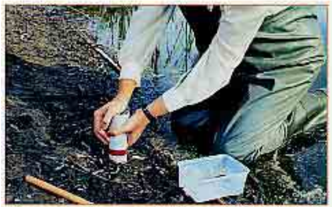
Taking a soil core with the corer.
