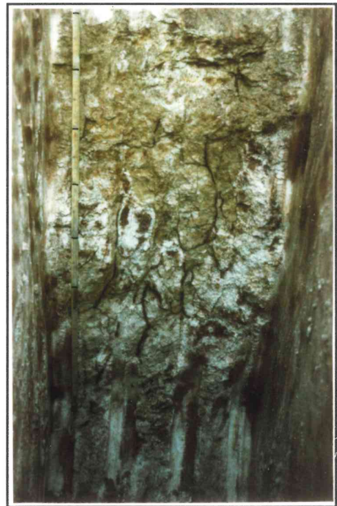
Figure 4: Subsoil of Soil A1. Exposed face showing how roots mainly occur along cracks and root channels (70 and 120 cm) in the clayey horizons of this soil. (Profile 91/MB1/E)
