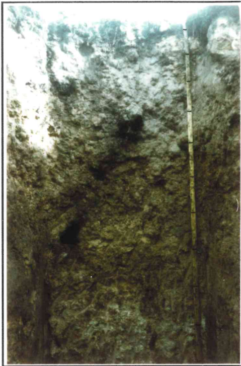
Figure 1: Soil A1 of the lateritised uplands. Note that the surface 60 cm is dominated by sand and ferruginous gravel, and although there are occasional boulders to 20 cm this soil does not have a pan. (Profile 91/MB1/L)
