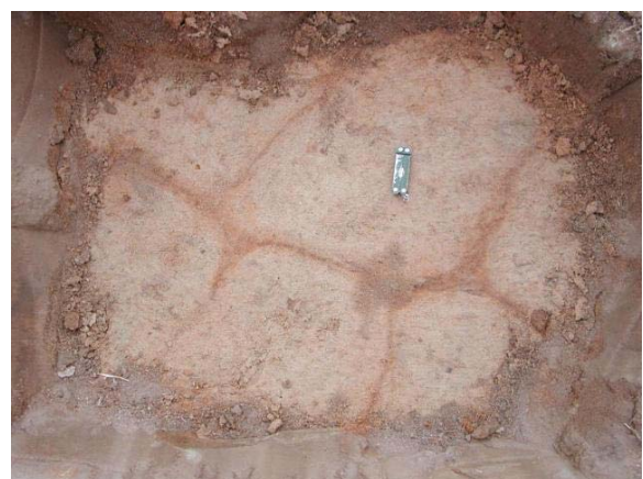
Figure 3: Lenses of porous material in clayey soil at Deluise site (Narembeen)
