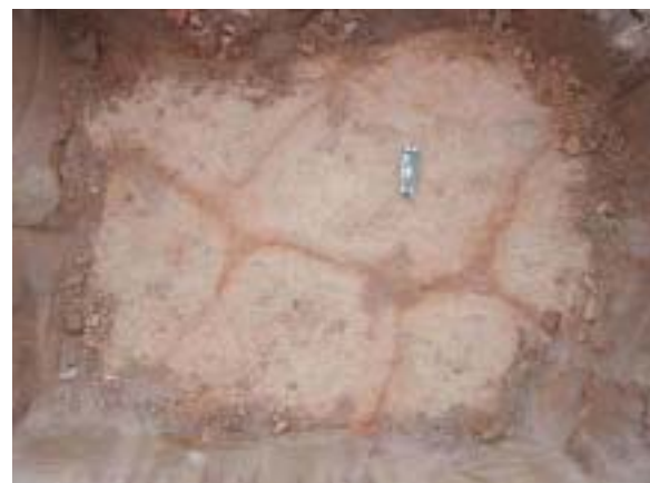
Figure 3: Lenses of porous material in clayey soil at Deluise site (Narembreen)
