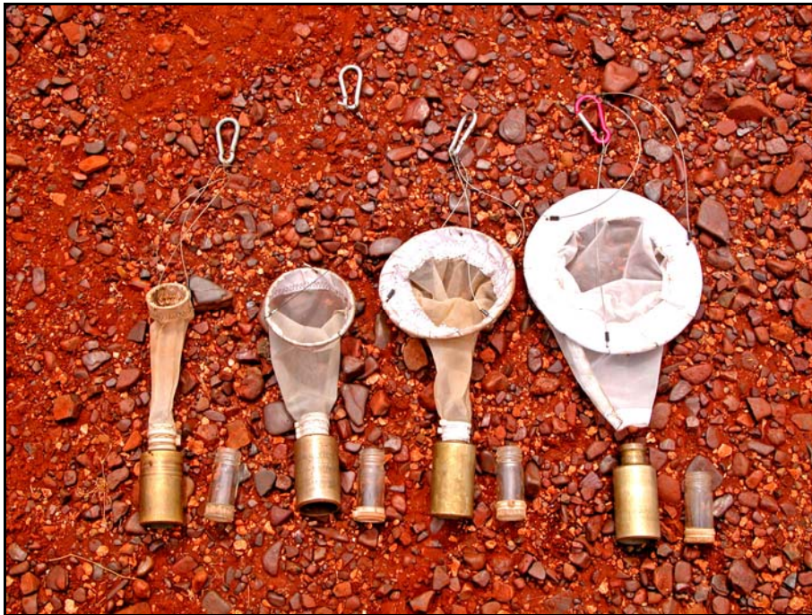
Fig. 3.1. Stygofauna nets of different diameters, showing the machined brass weight fitted to the bottom of the net and McCartney vial, with mesh base, that fits into the brass weight
