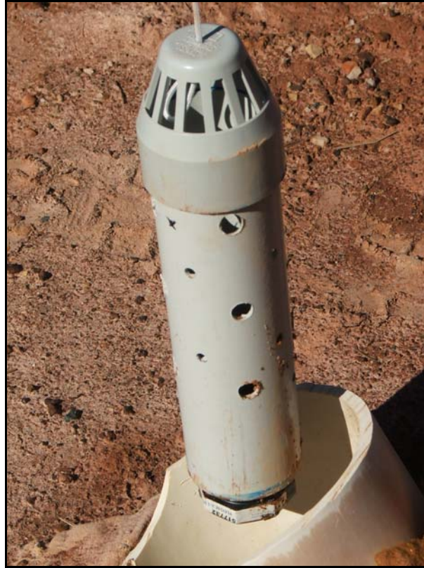
Fig. 3.2. Troglofauna trap being lowered into bore. Traps are made of PVC and ends are often closed with aviary mesh to provide access, rather than having holes drilled along the pipe
