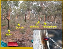
Measurements: Sapflow (heat ratio method), leaf gas exchange and water potential, local climate
