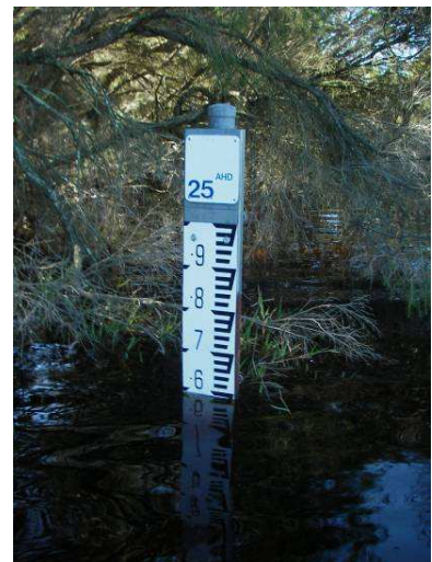
Photo 6: DoW depth gauge at Gibbs Road Swamp on 04Aug2008 read 24.59mAHD
