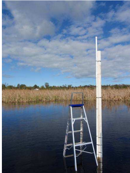
Photo 26: Water level logger, support tube and supporting angle iron. Nine Mile Swamp, 04Aug2009.
