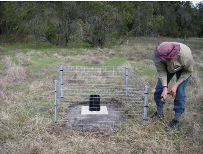
Photo 28: Tipping bucket rainfall recorders are being trialled on two SWWMP wetlands. Alan Clarke, 17Jun2009.
