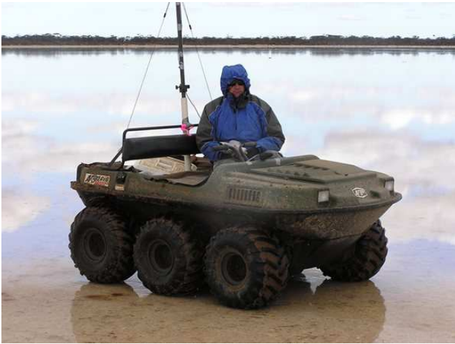
Photo 11: An amphibious vehicle is used to traverse the long distances involved in bathymetric survey of large dry or very shallow lakes. Steven Lowth, Lake Campion, 24May2004.
