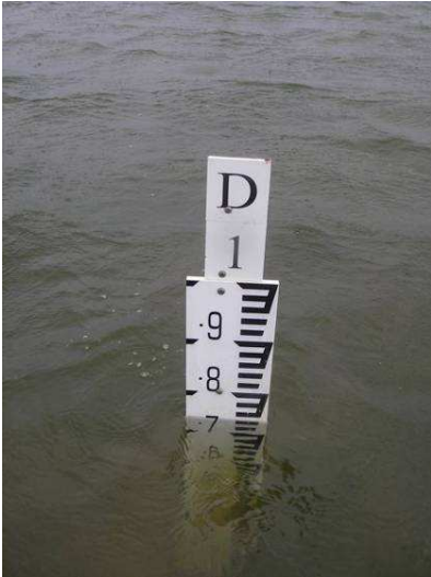
Photo 1: DEC depth gauge 'D' at Lake Muir on 18Sep2008 read 0.74m.
