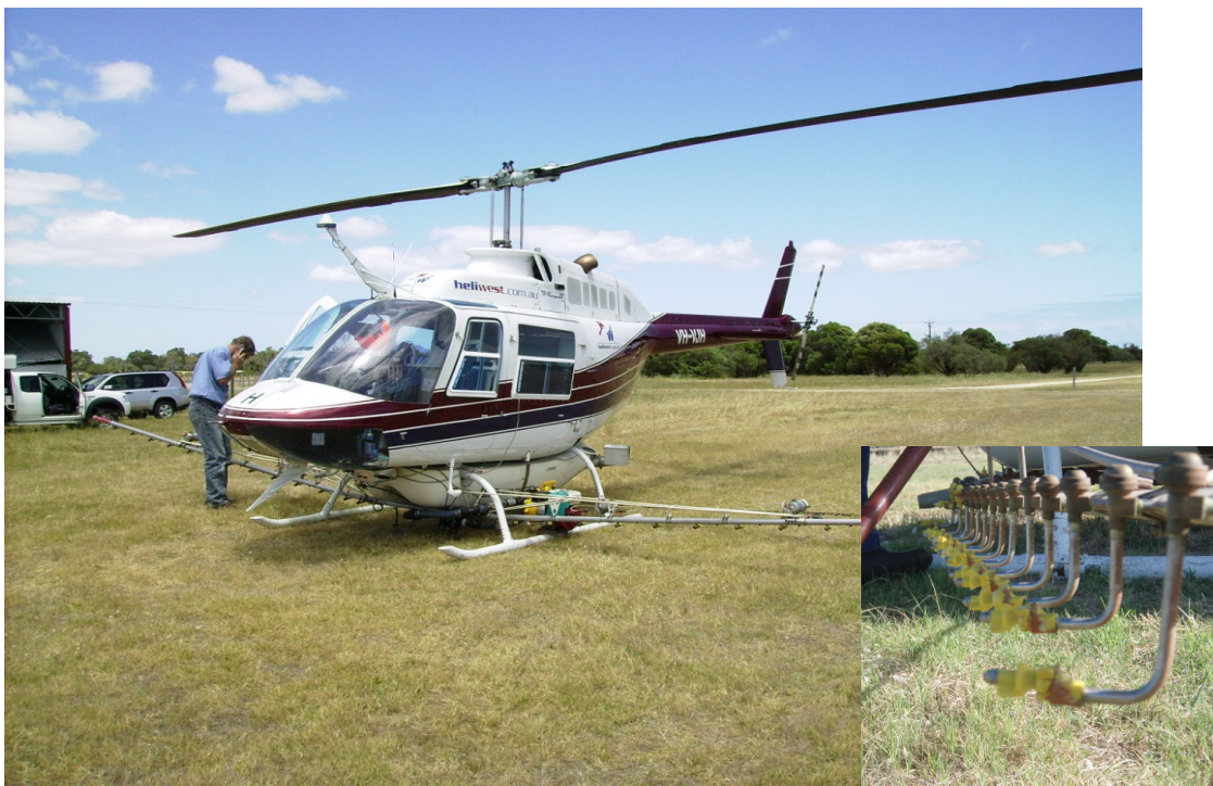
Figure 27: Helicopter fitted with liquid application equipment
