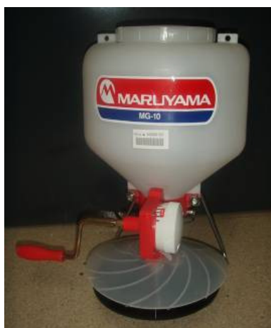
Figure 15: Hand operated granule spreader (Source: City of Mandurah)
