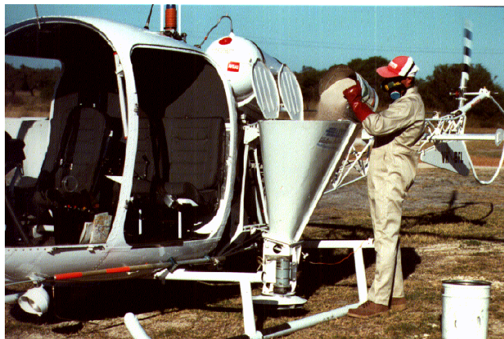
Figure 17: Mechanical hoppers being filled
