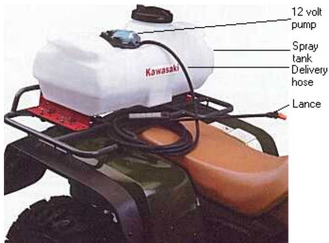
Figure 23: 12-volt sprayer mounted on ATV
