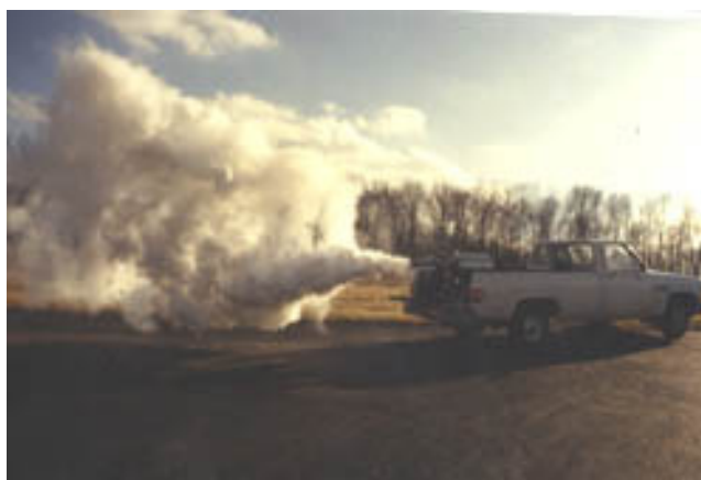
Figure 29: Vehicle mounted thermal fog unit in operation
