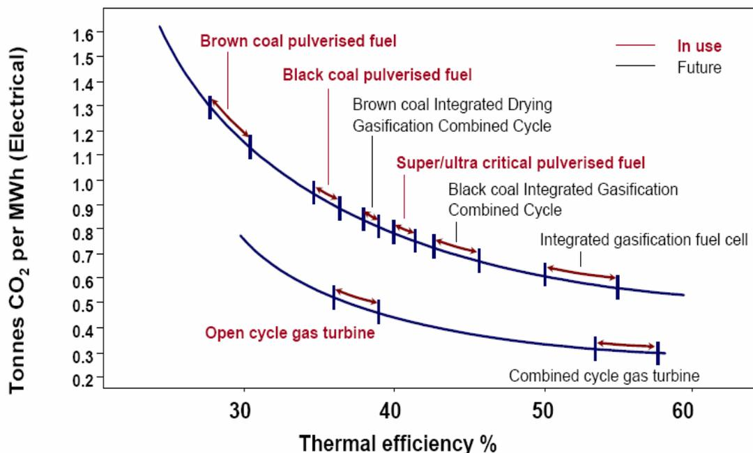
**Figure 6. Summary of CO<sub>2</sub> emissions and thermal efficiencies for coal-fuel processes.**
