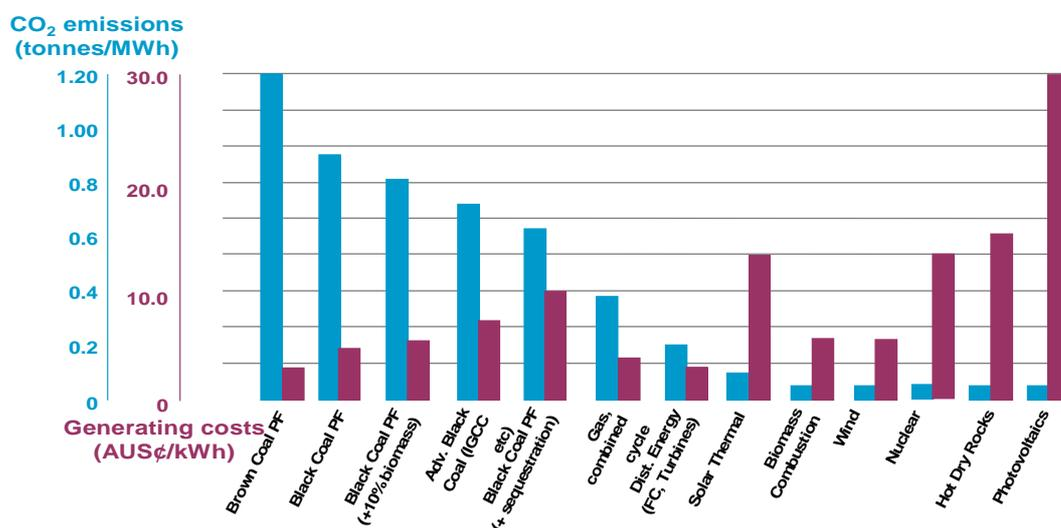
**Figure 11. Process generating costs and CO<sub>2</sub> emission comparisons**
