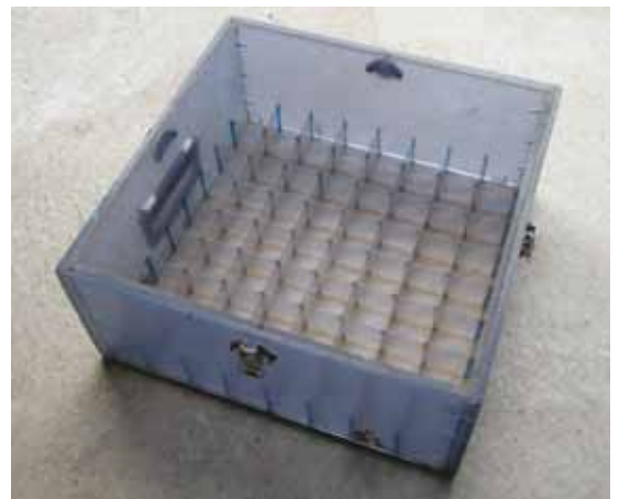
Figure 12. A box subsampler, shown with the lid removed. This one is constructed from perspex and measures 355 by 355 by 160 millimetres high. It contains 8 by 8 compartments, each 40 by 40 millimetres. 31
