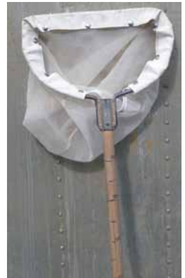
Figure 11. D-framed pondnet. The net opening is approximately 35 cm wide and 25 cm deep. The attached net is approximately 75 cm long.
