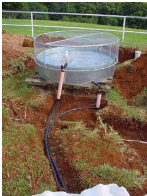
Figure 5. Class A evaporation pan. Image from Pickering (2007). 17
