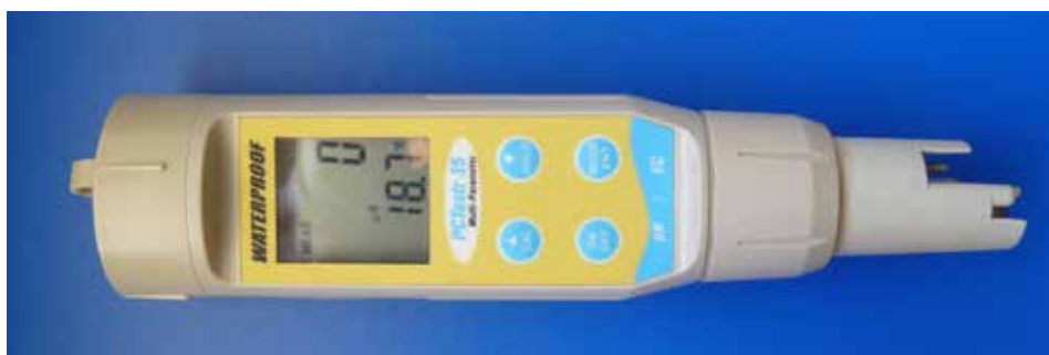
Figure 27. A meter that measures pH. Photo – J Lawn/DEC.
