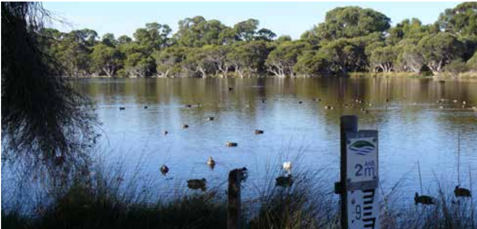
Figure 44. A staff gauge used to measure the level of inundation at Manning Lake, Cockburn. Photo – J Lawn/DEC.
