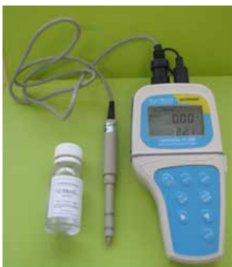
Figure 18. An electronic meter used to measure electrical conductivity in wetlands, with the probe attached and a solution used to calibrate the meter. This model also measures a number of other parameters. Photo – J Lawn/DEC.
