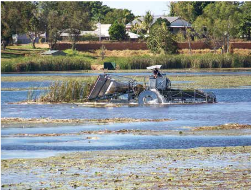
Figure 20. Aquatic weed harvester. Photo – K Tripp/Shire of Wyndham East Kimberley.
