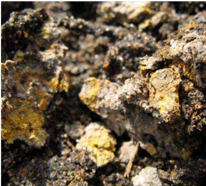
Figure 31. Jarosite is a butter or mottled orange coloured mineral that is a good indicator of actual acid sulfate soils as it only forms under acidic conditions.
