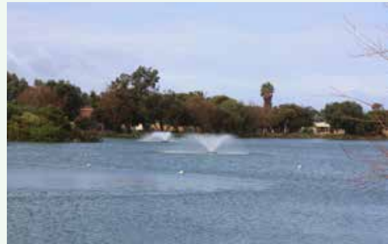
Figure 28. Bubbler (foreground) and fountains (rear) aerate the water and prevent anoxic conditions which can increase release of nutrients from the sediment and growth of algae and cyanobacteria. Photo - J Nichol/DEC.
