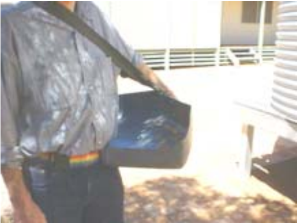
Figure 19. Seedling carrier with waist and shoulder straps. This carrier was designed specifically for open root plugs, ie seedlings are transferred from their cells to the carrier before planting.
