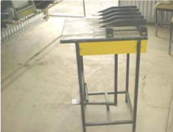
Figure 23. Automatic (foot operated) 'plug popping' device used in the nursery. Each tray takes about 4 seconds to be 'popped'.
