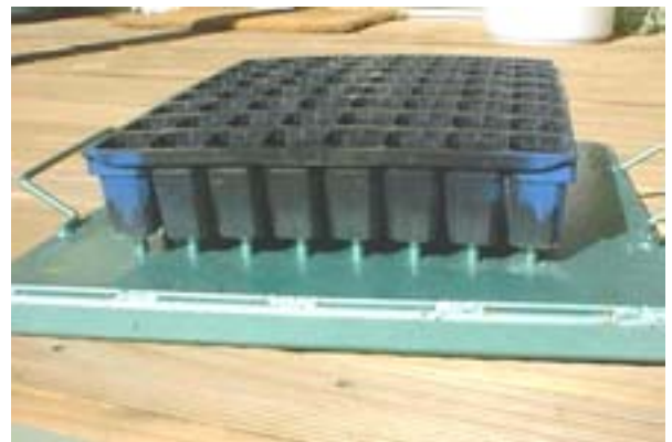
Figure 26. A manual 'plug popping' pad with seedling tray fitted part way down 'plug popping' position.
