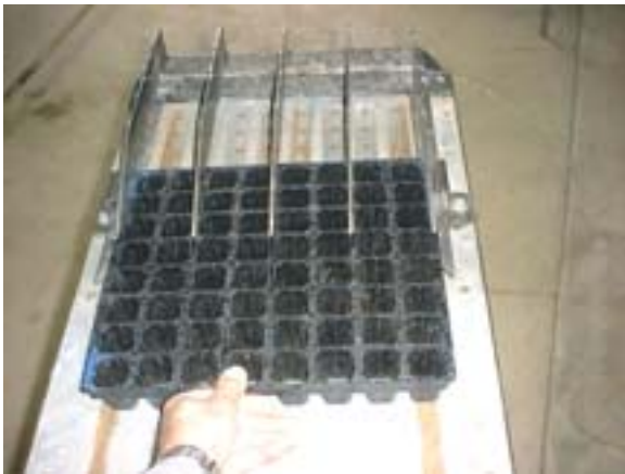
Figure 24. A tray being slid into position on the automatic (foot operated) 'plug popping' device.
