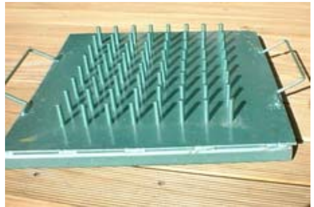
Figure 25. A manual 'plug popping' pad. This will allow 'plug popping' on-site if popping was missed during nursery dispatch or if circumstances necessitate on-site 'plug popping'.
