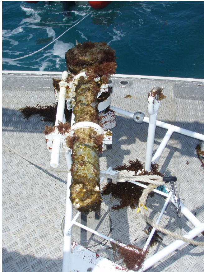
Figure 11 AQ2 mooring and bio-fouling after 6 week deployment
