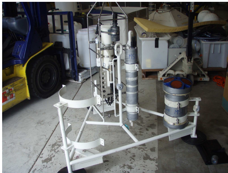
Figure 16 MS1 mooring showing SBE19p (left), SBE26 (middle) and RDI ADCP (right).
