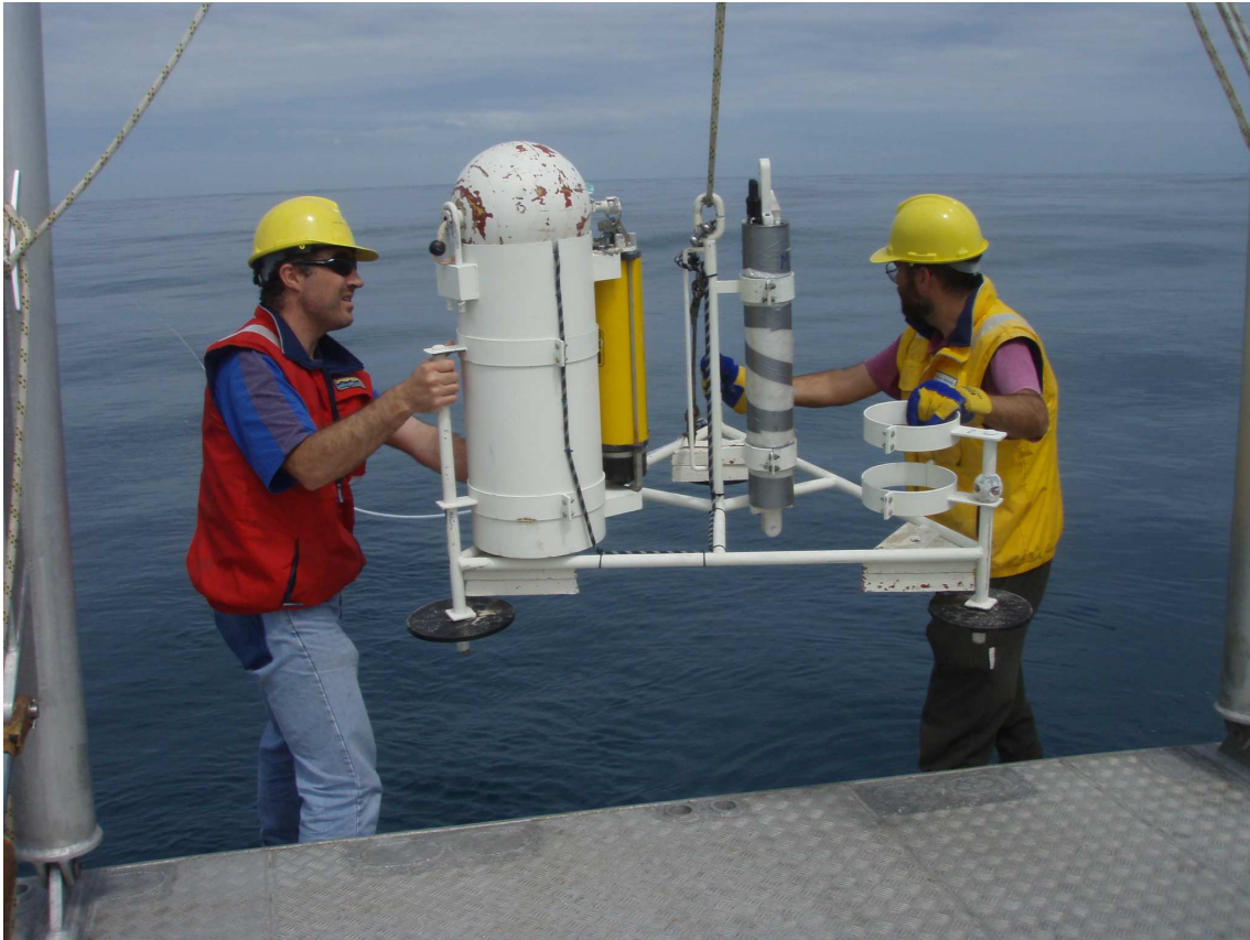
Figure 21 Deploying MS2 showing acoustic release and SBE26
