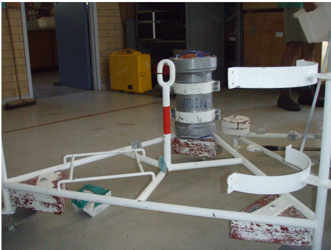
Figure 13 RDIN mooring frame with RDI ADCP
