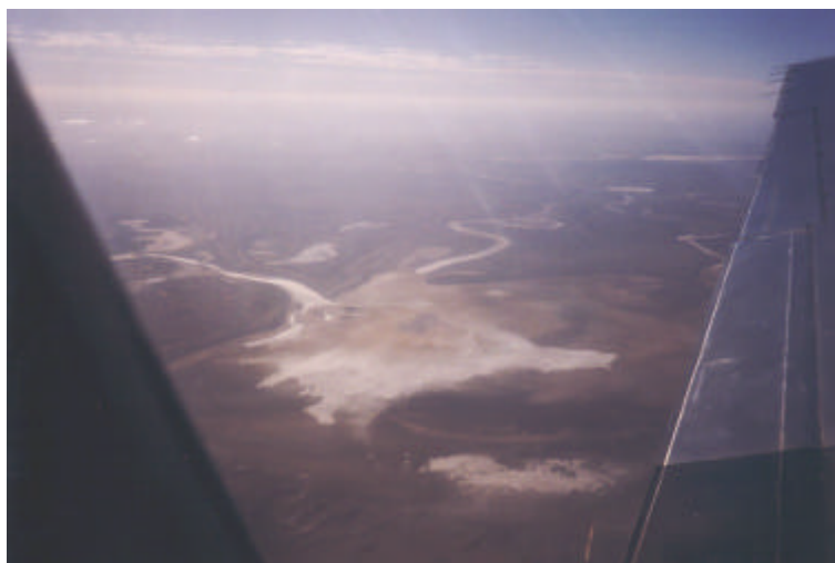
Figure 8. Evidence of surface salt on the lakebed surrounding the end of the discharge pipeline in April 2002, as seen from an aircraft. The visible salt is approx. 2 km in diameter (S. Vellekoop, 2002).
