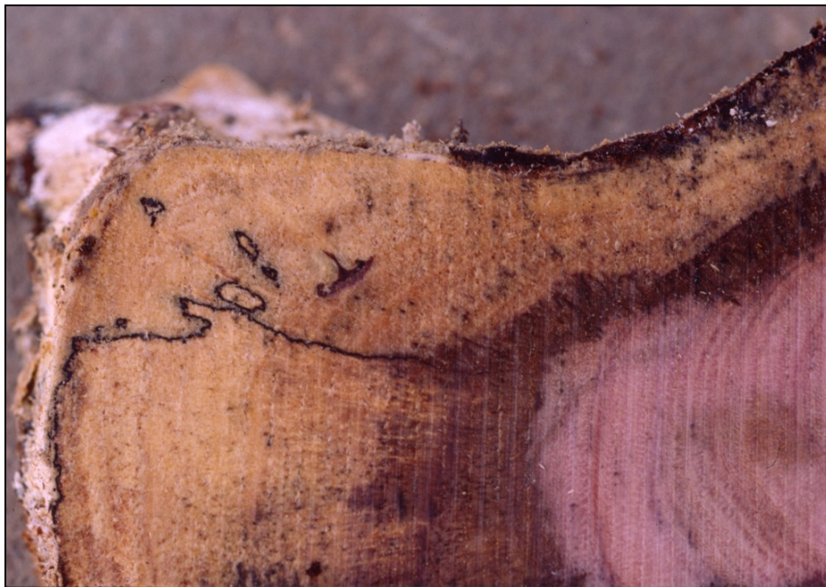
Above: Typical white rot and zone lines in infected wood
