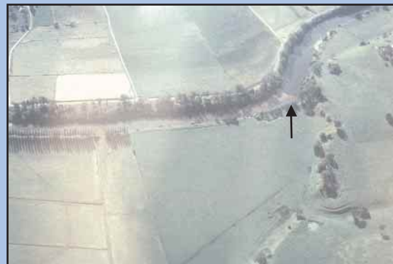
Figure 59. The front of the sand slug in the Tambo River (see arrow) (the water is about 5 m deep downstream of the front of the slug).
