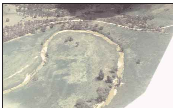
Figure 57. Sand aggrading the Lachlan River (New South Wales) originating from historical gully and sheet erosion.
