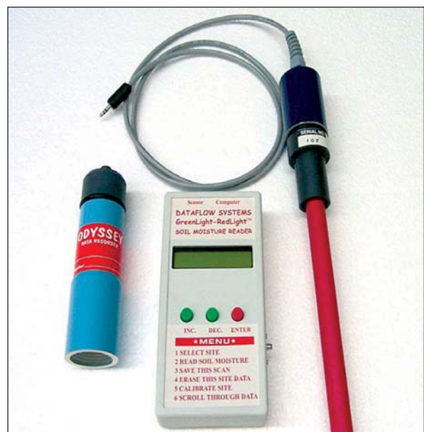
Figure 14. GLRL portable or in situ soil moisture sensor and logger/handheld reader.
