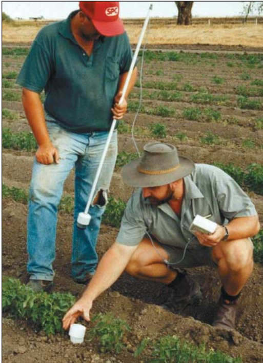
Figure 13. Gopher is a manually operated soil moisture monitor.
