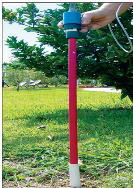
Figure 14. GLRL portable or in situ soil moisture sensor and logger/handheld reader.
