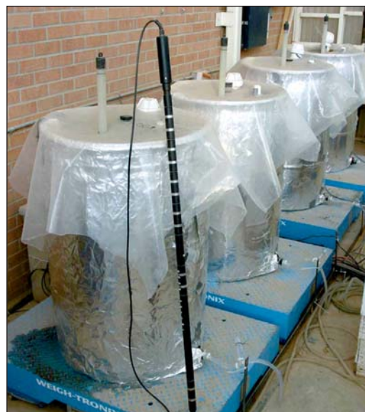
Figure 43. Soil columns on scales. Columns were 55 cm in diameter and contained a soil depth of 75 cm. Sides of columns were covered with aluminum foil to reflect radiant energy. Columns were covered with plastic sheeting after saturation. In foreground is the Delta-T PR1/6 capacitance probe.
