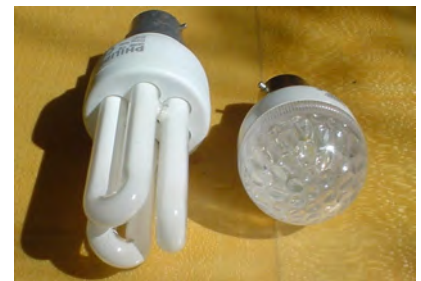
Figure 9.4. Philips 11 W alongside Omicron 1.3 W LED bulb.
