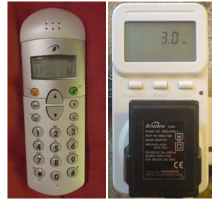
Figure 11.3. This wasteful cordless phone and its charger use 3 W when left plugged in. That’s 0.07 kWh/d. If electricity costs 10p per kWh then a 3 W trickle costs £3 per year.
