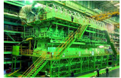
Figure A.15. The Wartsila-Sulzer RTA96-C 14-cylinder two-stroke diesel engine. 27 m long and 13.5 m high. www.wartsila.com
