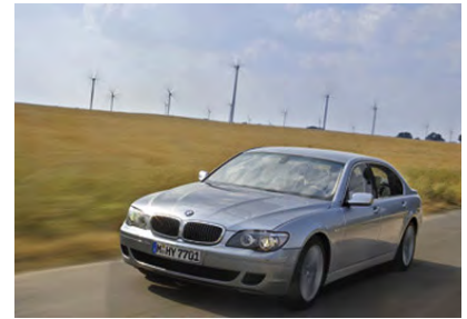
Figure 20.26. BMW Hydrogen 7. Energy consumption: 254 kWh per 100 km . Photo from BMW.
