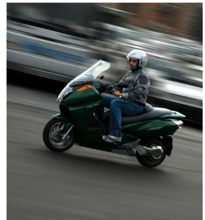
Figure 20.44. Vectrix: 2.75 kWh per 100 km . Photo from www.vectrix.com .
