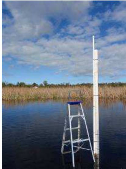
Photo 26: Water level logger, with support tube and angle iron. Nine Mile Swamp, 04Aug2009.
