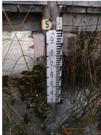
Photo 5: DPaW depth gauge 'C' at Lake Clifton on 13Sep2008 read 4.30m.
