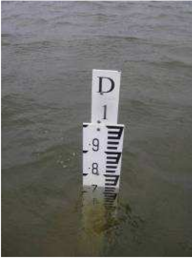
Photo 1: DPaW depth gauge 'D' at Lake Muir on 18Sep2008 read 0.74m.
