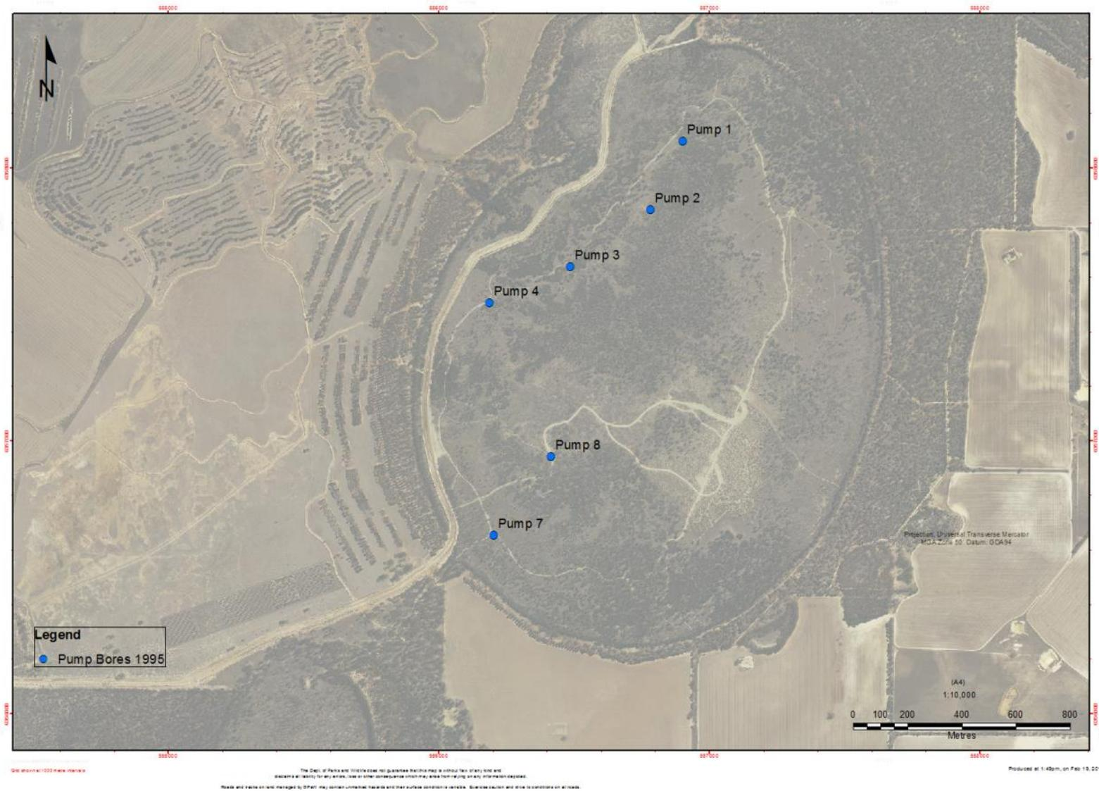
Figure 6: Pumping bores installed in the Toolibin Lake NDRC 1999
