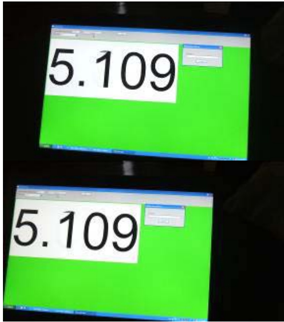
Figure A 2: Images showing the process of checking the synchronisation of the camera. The two images represent the left and right images captured by the FUJI camera.
