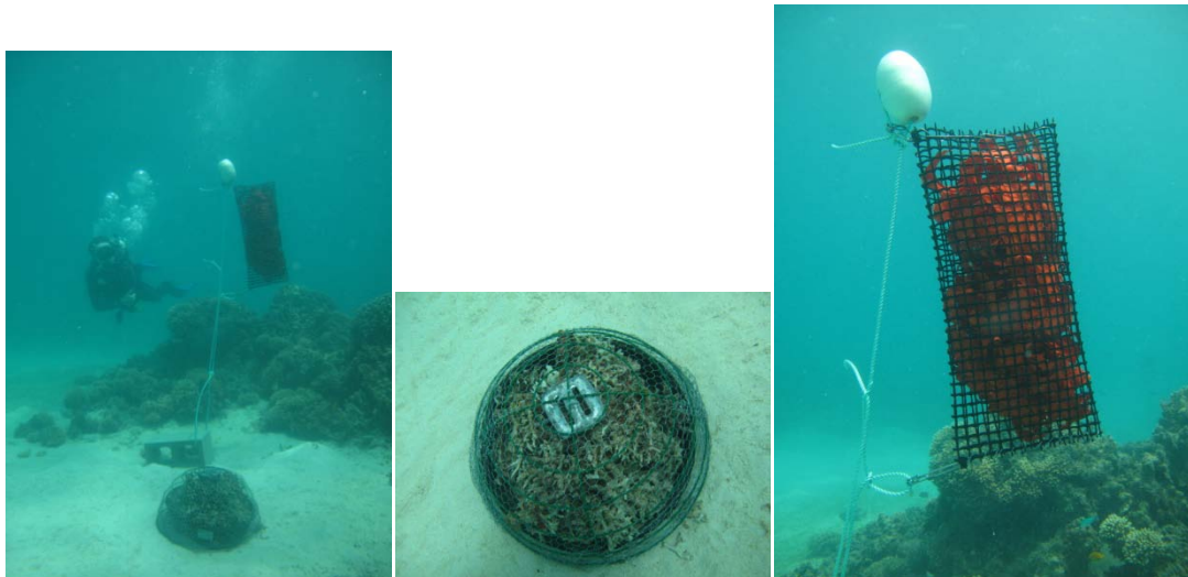
Figure 18a-c: a) Benthic and mid-water fish aggregation devices trialed and deployed to ensure that as wide a range of species as possible was included in juvenile fish counts. b) benthic design of plastic sieve filled with coral rubble and protected from medium and large predators with wire. c) mid-water SMURF design made of plastic barrier fencing encased in a hard plastic gutter guard mesh.
