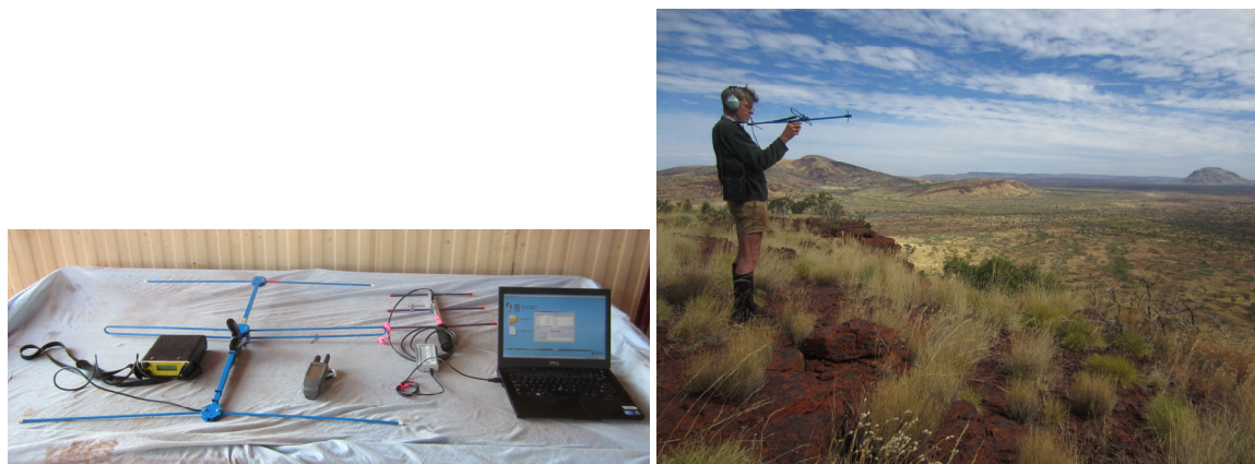
Figure 10. (a) VHF radio-telemetry receiver and Yagi (left) and UHF Yagi and modem used to undertake remote download of Telemetry Solutions GPS collars (right). (b) Radio-tracking from a hill top.
