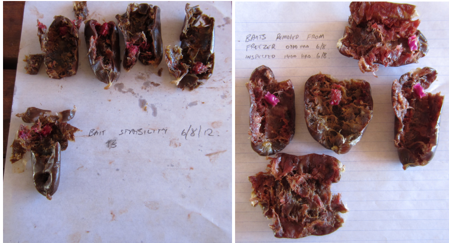
Figure 13. (a) Baits removed from the weathering cage. Note the dye-stained meat adhered to the pellet (b) Baits withdrawn from the freezer and assessed on same day.
