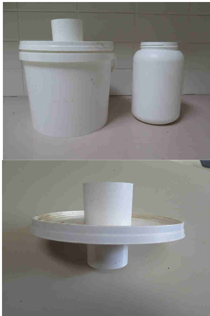
Figure 22a: (top) showing the difference in dimensions between a standard trap (right) and modified traps (left) and Figure 22b: (bottom) showing the position of the PVC aperture tube in the lid for the modified trap.
