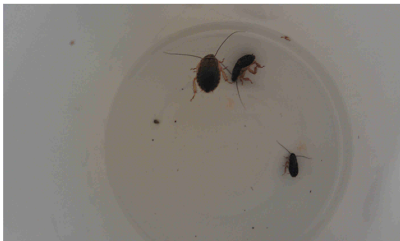
Figure 18: Cockroach “test subjects” were introduced to the trap containing 70% ethanol and 30% propylene glycol
